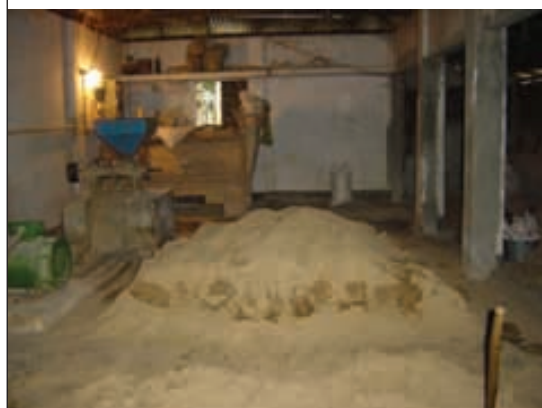
FIGURE 3 Ground mixed feed ingredients ready for pelleting in a small pellet machine
