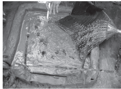
Testing different outflow designs under different rainfall intensities Photo: SUFA
