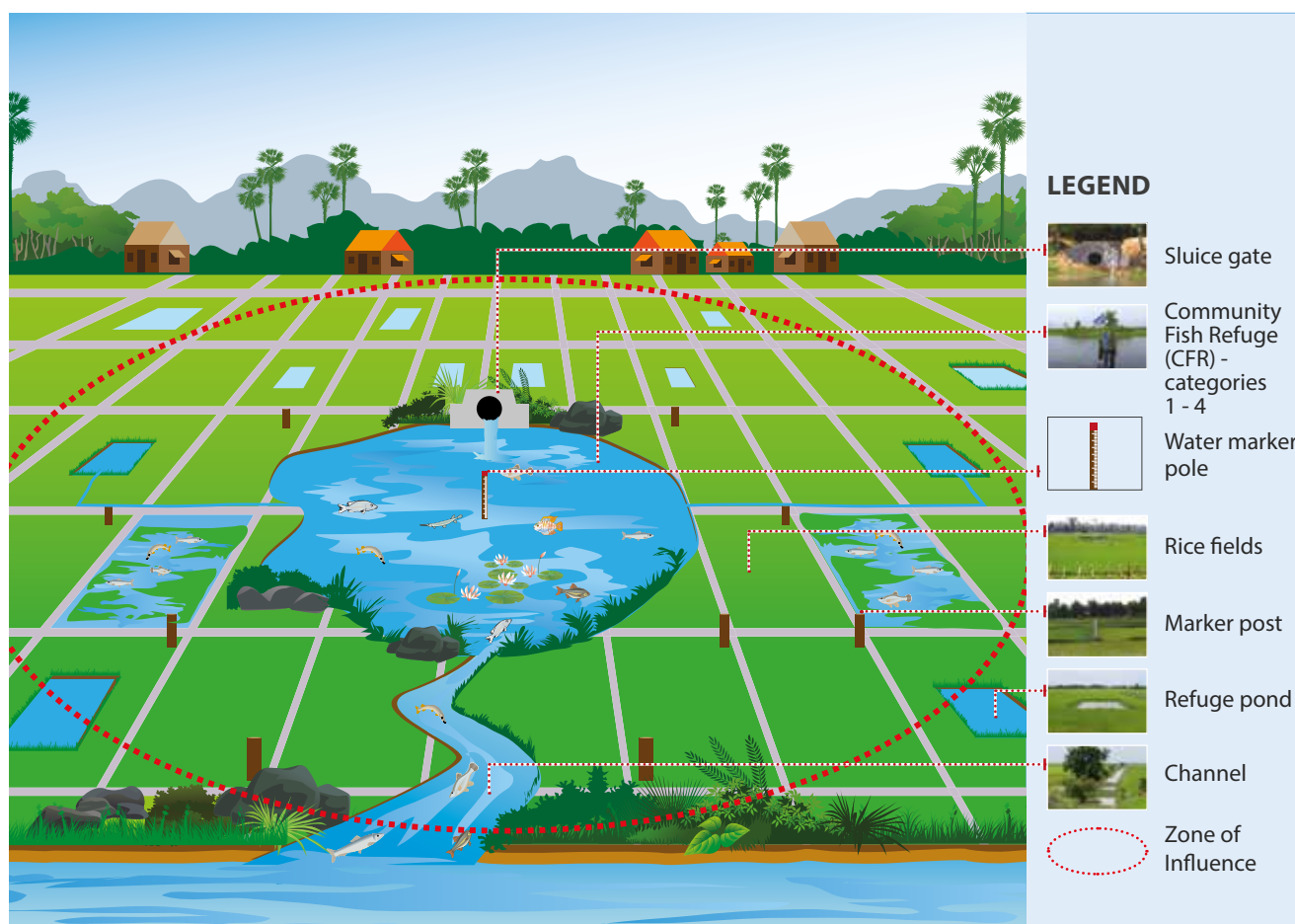
Chart 1: the main physical components of the Rice Field Fisheries / Community Fish Refuge system (see text on next page for CFR category descriptions).
