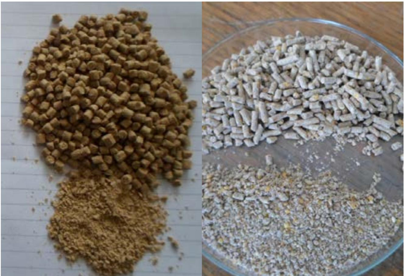
**Figure 14:** Compressed fish feeds produced by the private sector. Left: good quality feed. Note the size homogeneity of the pellets and the well-ground ingredients. Right: bad quality feeds. Note the variation in pellet sizes with some very large pellets (over 1 cm long). Note also the poor grinding of the ingredients with unground large pieces of yellow corn. Courtesy: A.-F.M. El-Sayed.
