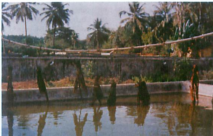
Sugarcane bagasse tied to bamboo beams for suspension in experimental cisterns.
